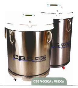
CBS Isothermal Freezers feature a patented liquid nitrogen jacket to provide uniform storage temperatures in the -190°C range, free from liquid nitrogen contact. This innovative design eliminates the risk of cross-contamination through liquid nitrogen and the need for additional packaging to protect valuable cells and tissue.
